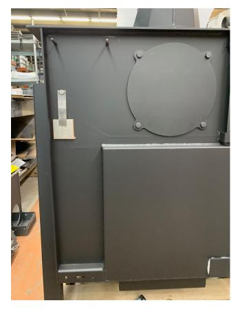
3. Use a 7/16" wrench or socket and remove the hex head bolt that holds the tertiary air damper to the back of the stove. Keep the bolt for the new installation.
